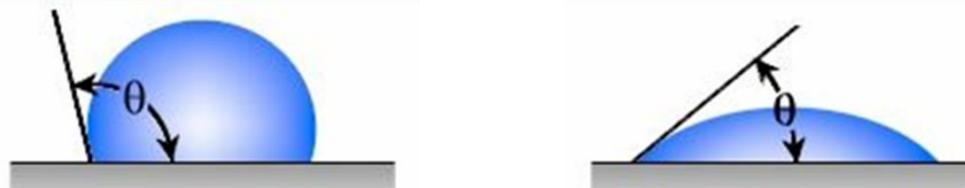
Figure 4: Explanation of Contact Angle and Hydrophobicity
